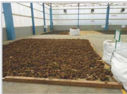
Dewatering of sludge using solar energy
