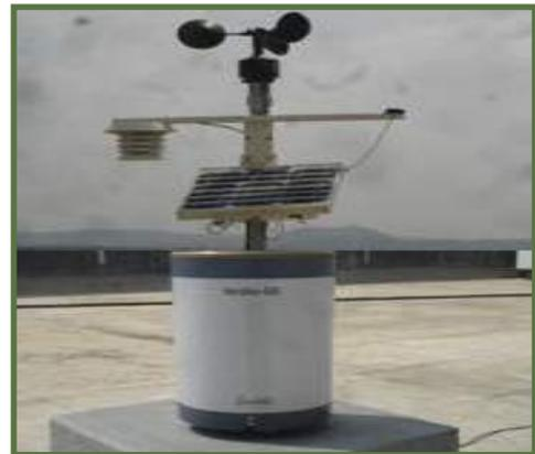
Fig 6.7: Weather Monitoring Station
