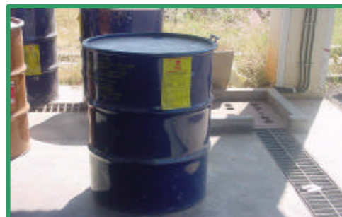
Hazardous waste are filled in MS drums, labeled & stored at Hazardous waste storage Yard.
